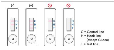
Any reading after 12 minutes from the initial application of the sample into the 3M Bovine Total Milk Protein LFD should be considered invalid. A reading at this time cannot be interpreted and can lead to erroneous results.
