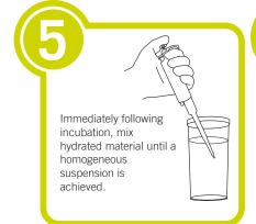
Proceed with the challenge according to laboratory protocol. The challenge must be completed within 30 minutes of the hydration process to avoid a change in the challenge suspension concentration.
